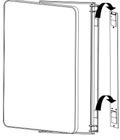
2. Mount wall plate by latching upper and lower slots on wall plate onto back plate on wall
